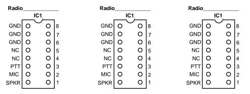
[] Following your diagram, carefully install the jumpers at IC1.
